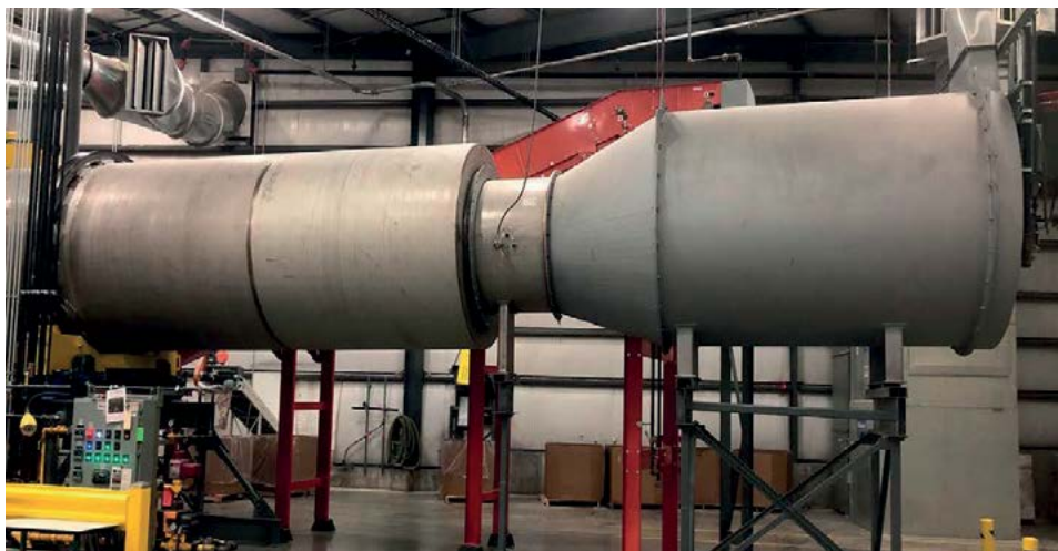
Rotary dryer with combustion chamber.
