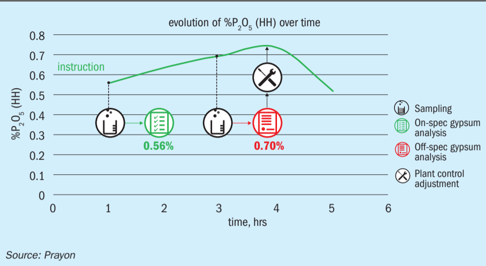
Fig. 2: Delays in process control due to the interval between sampling and time taken for subsequent laboratory analysis ( \% P_2O_5 ) of hemihydrate cake quality
