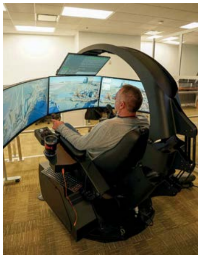
Cover: State-of-the-art remote operation station at Mosaic's Integrated Operations Center, Lithia, Florida. The operator is controlling high-pressure water guns in the phosphate mining area miles away. Photo: The Mosaic Company.
