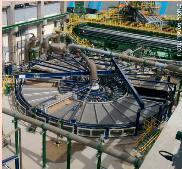
Above: Profile’s model 30-220 tilting pan filter with a total surface area of 220 m 2 . Installed at OCP’s Jorf Lasfar phosphates production complex in Morocco.
