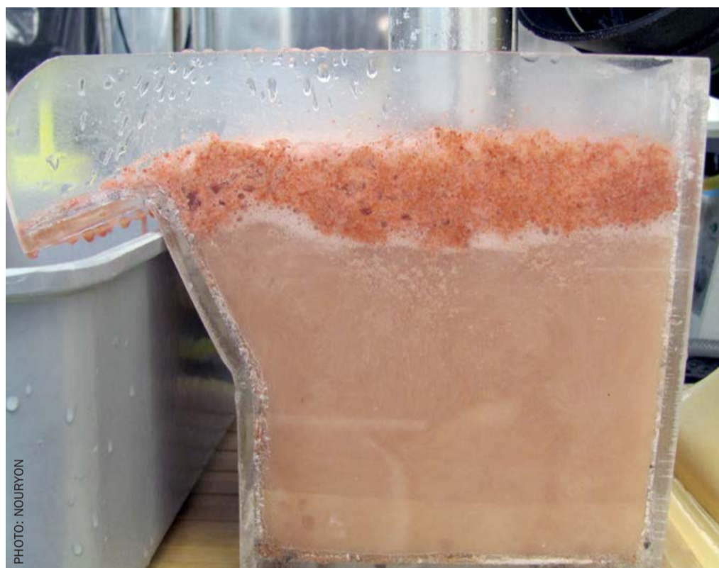
Typical sylvite flotation test in Nouryon's application lab.
