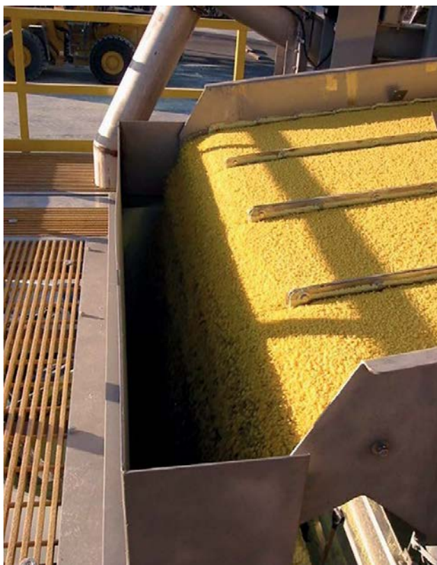
Below: The formed sulphur prills from the Devco II system after screening.
