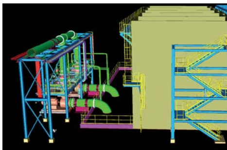
Fig. 5: Cooling water pumps – installed at ground level.
