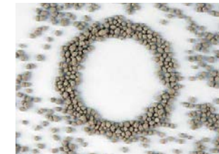
Polysulphate Premium is granulated from powdered polyhalite to form uniform, robust spheres.
