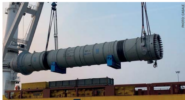
Two massive pieces of revamping equipment – an ammonia converter and BFW preheater – being loaded onto a US-bound ship in Venice at dawn.
