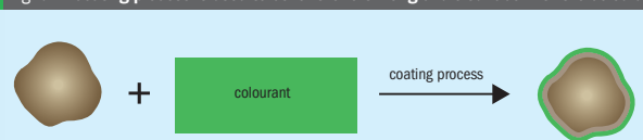
Fig. 5: A coating process is used to cover the fertilizer granule surface with the colourant
