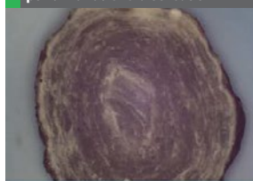
Fig. 6: Cross-section of a single fertilizer granule at different magnifications showing colourant performance and distribution
