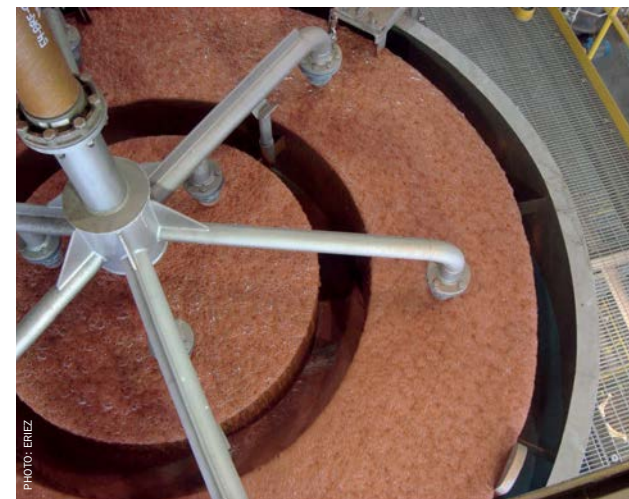
The generation of a deep froth by an Eriez ® CavTube ® column flotation cell helps to improve the flotation of fine potash.
