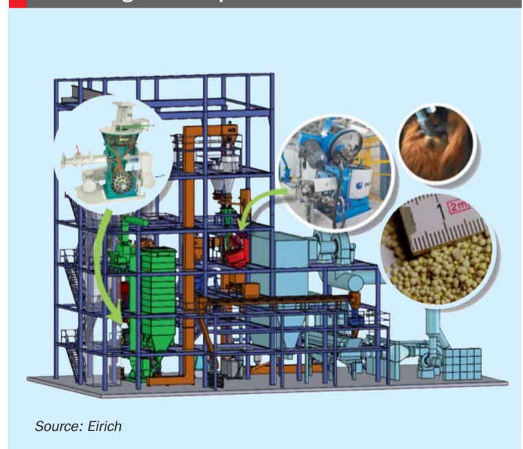
Fig. 2: EIRICH SmartMixer within a fully automated mixing and granulation plant
