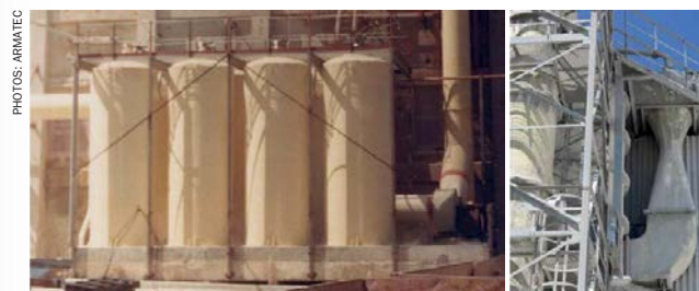
Traditional void towers (left) struggle to meet today's strict emissions limits. Venturi scrubbers (right), while a common solution, also have several limitations.
