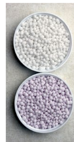
Urea granules: uncoated (top) and coated (bottom).
