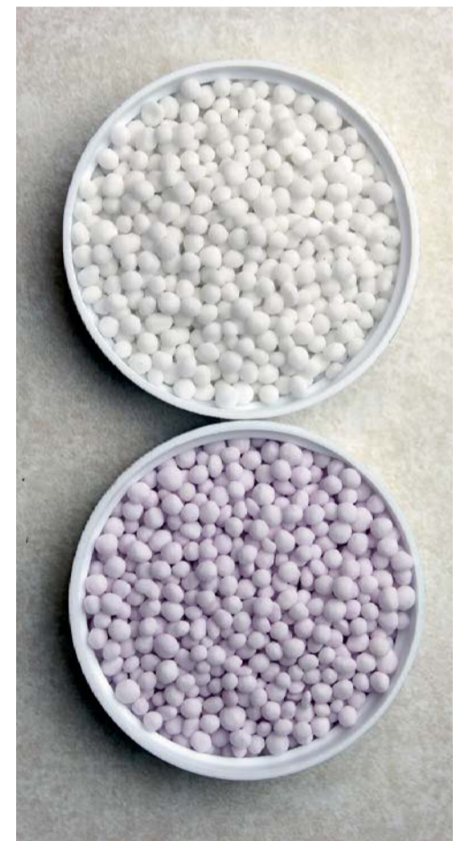
Urea granules: uncoated (top) and coated (bottom).
