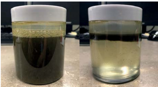
Fig. 3. Jar testing is crucial for revealing how blends will behave over the long-term in the field. In this example, the blended ingredients were compatible at initial mixing (left) but showed strong separation after sitting for 48 hours (right). This shows a clear failure that should be avoided.
