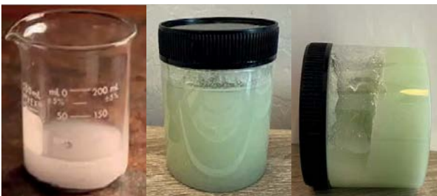
Fig. 2. When mixed, incompatible liquid fertilizers can form solid precipitates (left photo) that can damage and clog equipment. In another example, a jar test revealed that liquid calcium fertilizer (calcium ammonium nitrate) is severely incompatible with a phosphate-based fertilizer (ammonium polyphosphate) as they form an immobile green sludge when combined (centre and right photo). This blend would have caused considerable headaches if formulated on a large scale.
