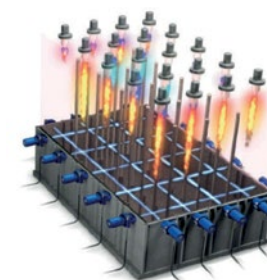
Fig. 4 Laser grid distribution on a down-fired reformer, paths depicted to each measure temperature O 2 , CO, CH 4 and H 2 O and provide a distribution of combustion in the heater.
