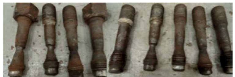
Fig. 6: Corroded carbon steel bolts.
