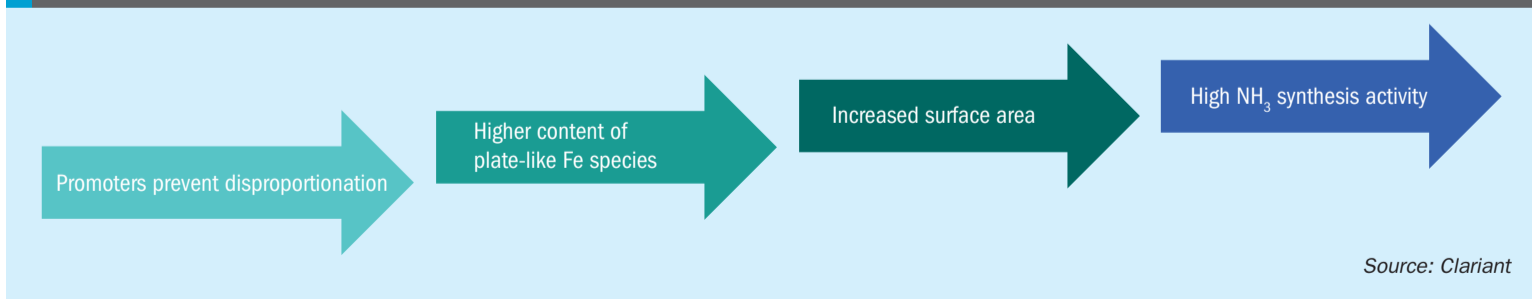
Fig. 5: Scheme illustrating the impact of promoters on activity based on the proposed reduction mechanism
