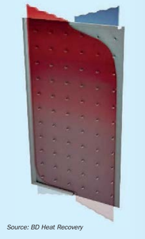
Fig. 3: Counter flow heat exchanger
