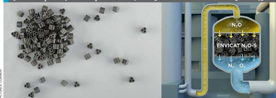
Fig. 1: EnviCat N 2 O-S catalyst removes N 2 O from nitric acid plant tail gas and converts it into harmless nitrogen and oxygen
