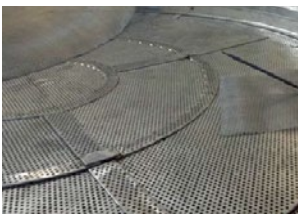
Fig. 6: Inside of a basket in good physical condition and with an even and level support.
