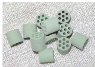
Fig. 2: Leading secondary N_2O abatement catalyst Yara 58-Y1.
