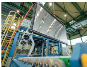
Assembly of the thyssenkrupp Nucera electrolyzers at Camacari.
