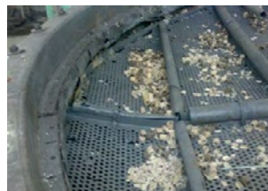
Fig. 7: Inside of a basket in poor physical condition and with an uneven support.
