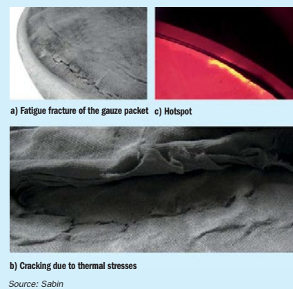
Fig. 3: Influence of flow effects on the catalyst
