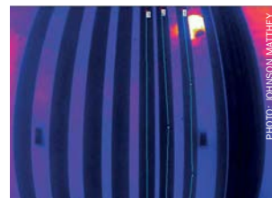
Fig. 6: Still image from video recorded by Reformer Imager, showing sections of reformer tubes.
