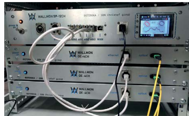
Fig. 1: Optoelectronic unit responsible for interrogation of fibre-optic sensors and online signal processing.
