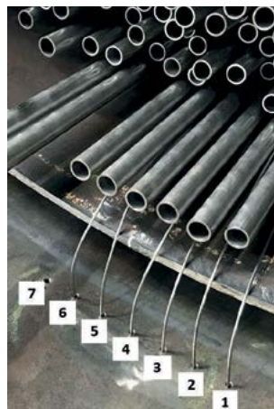
Fig. 5: Integration of ultrasound sensors into the CO 2 stripper.
