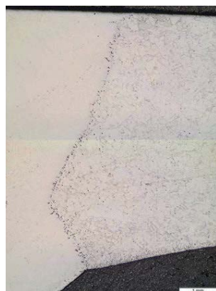
Fig. 7: Creep voiding observed along the fusion line of a pigtail weld joint
