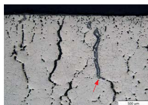
Fig. 6: Example of stress relaxation cracking in an Alloy 800H/ Alloy 800HT pigtail, highlighted by the red arrow. Creep voiding and cracking is also shown.
