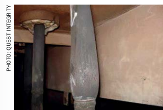
Fig. 3: Observed diametral expansion of a pigtail
