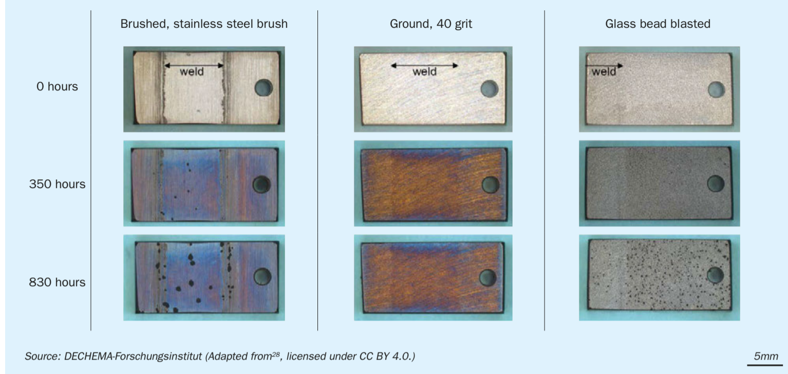
Fig 1: Weld beads of alloy 602 CA with three industrially applied surface treatments: brushed, ground, or glass bead blasted exposed in harsh laboratory metal dusting environments.
