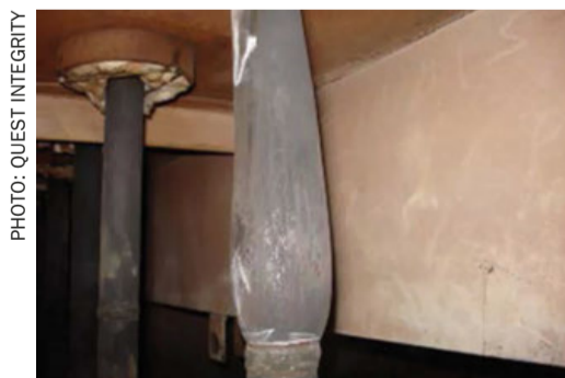
Fig. 3: Observed diametral expansion of a pigtail
