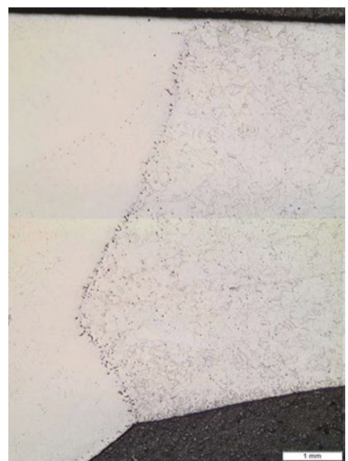
Fig. 7: Creep voiding observed along the fusion line of a pigtail weld joint
