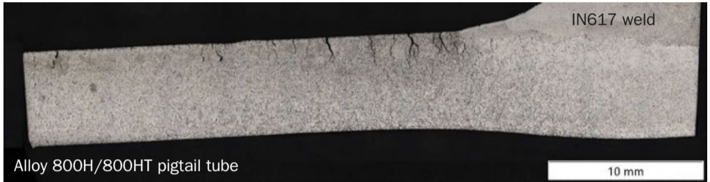
Fig. 4: Example of a mixed grain size distribution and the corresponding circumferential creep damage observed. Average ASTM grain size = 2.99. Evidence of bending is also shown in the pigtail cross section.
