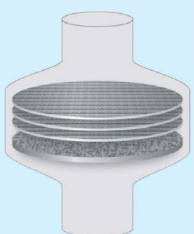
Fig. 2: Ammonia converter in a nitric acid plant with primary and secondary catalyst
