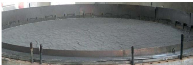
PGM catalyst in a nitric acid plant.
