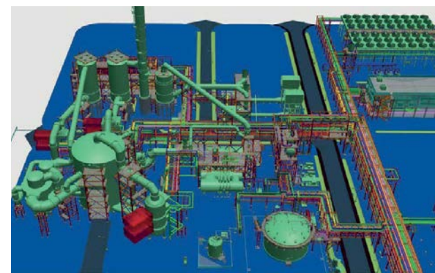
3D model of a large acid plant (no HRS) in a fertilizer complex.
