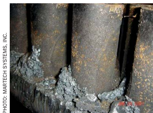
Fig. 1: FAC on condenser Inlets (high purity BFW)
