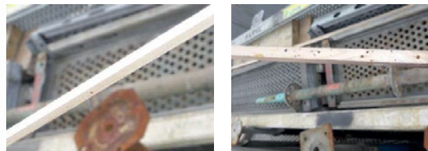
Fig. 3: Drying tower stick tests. Left: clean. Centre: Some carryover. Right: Severe carryover.
