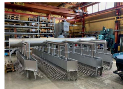
Fig. 9: Edmeston SX® alloy distributors from Metso Outotec. Left: FIDi European Patent EP 2 173 464 B1. Centre: Lurgi deflector plate. Right: Trough type.
