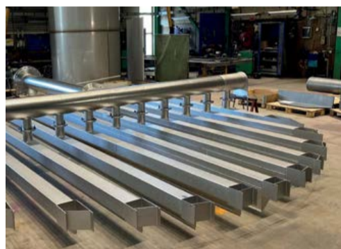
Fig. 9: Edmeston SX® alloy distributors from Metso Outotec. Left: FIDi European Patent EP 2 173 464 B1. Centre: Lurgi deflector plate. Right: Trough type.
