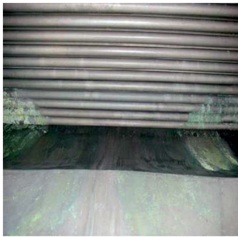
Fig. 4: Sulphate formation on shell side of cold reheat exchanger.
