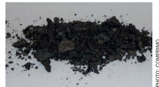
Fig. 4: No. 1 reheater process (shell) side deposits.
