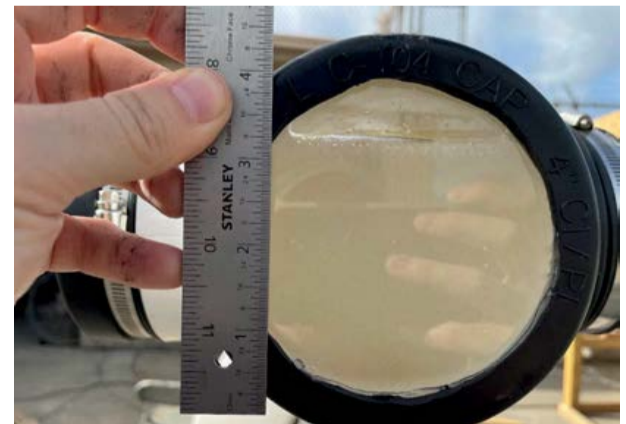
Left: Example of liquid level rise at entrance to horizontal elbow fitting. Right: Example of liquid level viewed through sight glass on elbow.
