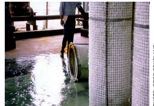
Fig. 2: Removed candle filters contaminated with \text{NO}_x .
