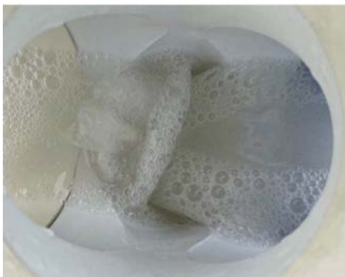
Example of liquid flow through the vertical drop; view from above.
