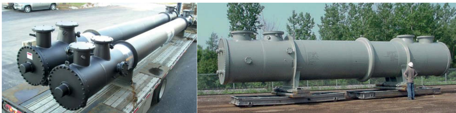
Fig. 3: The increasing size of acid coolers. Left: 800 t/d plant, 0.8 m shell ID, 5.3 m 3 acid, 2.4 m 3 water. Right: 4,400 t/d plant, 1.8 m shell ID, 18 m 3 acid, 7.5 m 3 water.
