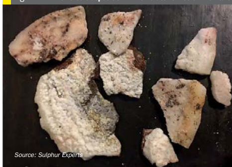
Fig. 12: Ammonia salt deposition in incinerator emission monitors
