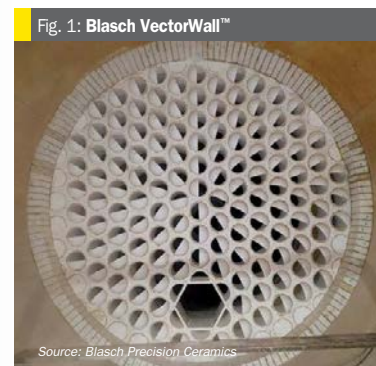
Fig. 2: Improved mixing with a VectorWall™
