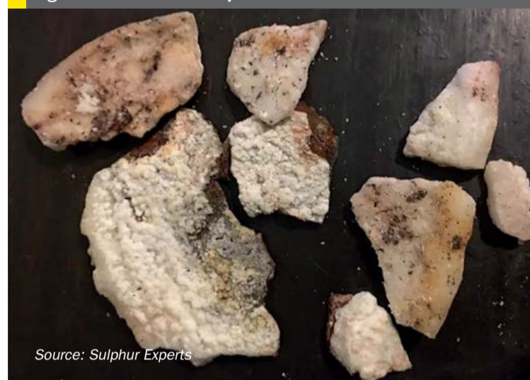
Fig. 12: Ammonia salt deposition in incinerator emission monitors
