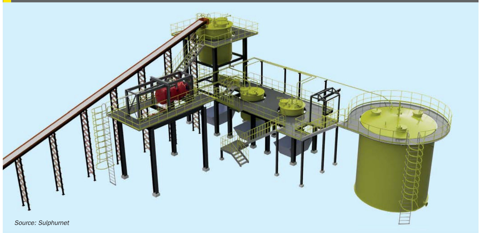
Fig. 1: Sulphur melting and filtration plant
