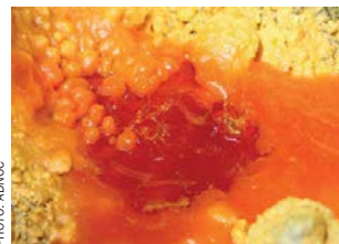
Fig. 1: Molten sulphur at temperatures >155°C.
