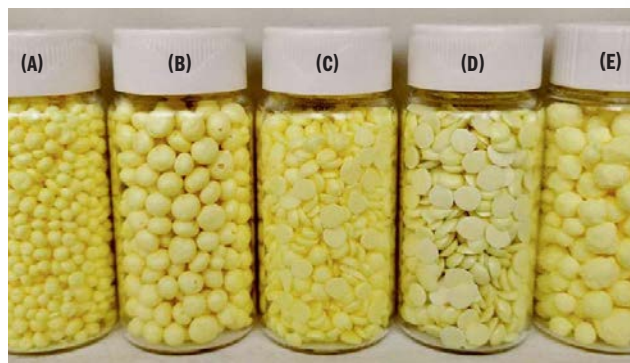
Fig. 1: From left to right: (A) commercial air prills, (B) lab formed water prills, (C) commercial pastilles, (D) lab formed pastilles and (E) commercial granules.
