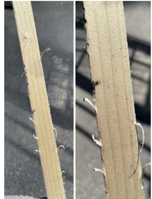
Fig. 5: Clean stick test results from J. R. Simplot's IPAT installation of PI fibre beds at 18 months of service.
