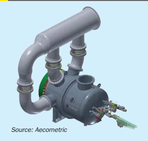
Fig. 1: 3rd generation incinerator burner configuration
