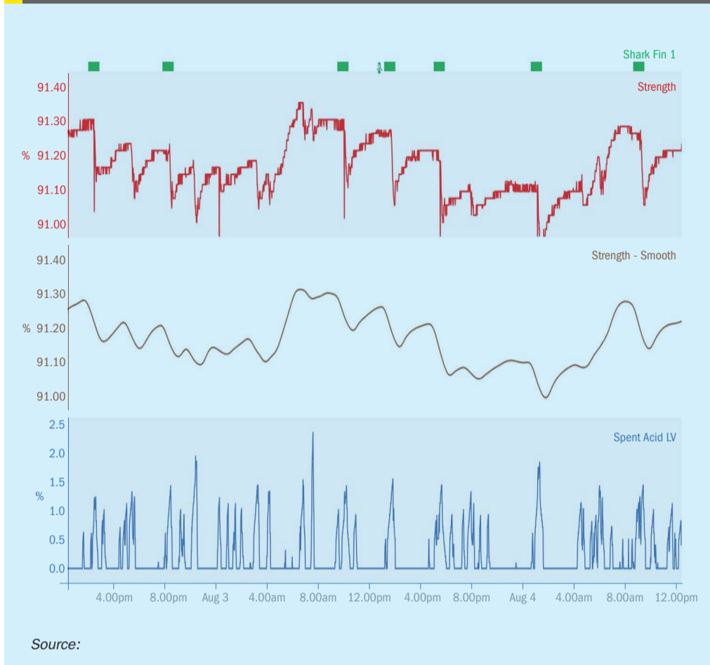
Fig. 2: Raw data, smoothed data and suspected root cause (valve position) trends to build shark fin pattern detector (condition) using Seeq® Workbench which is an embedded tool in the MECS® digital advisor. Green bars at top indicate a pattern detected (capsules).
