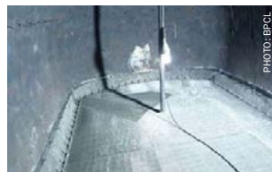
Fig. 9: Bottom grid after mesh modification
