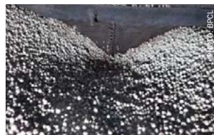
Fig. 6: Pit near mesh-catalyst interface
