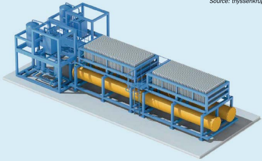
Fig. 2: Modular, skid-mounted thyssenkrupp water electrolysis unit
