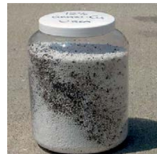
Fig. 1: Uneven micronutrient fertilizer distribution (left) in a bulk fertilizer blend. The patchy distribution of granular copper oxy-sulfate (dark) within the urea (white) is clearly visible. This contrasts with the even distribution of a copper dry dispersible powder (right). Every urea prill in the blend is coated with copper.
