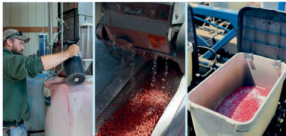
Fig. 2: Applying nutrients to seeds as a liquid coating via a commercial seed treater (left). Nutrients can also be applied dry via a powder additive feeder as a seed finisher (middle). Dry nutrient powders can also be added directly in a seed planter box as a coating and seed flow aid (right).
