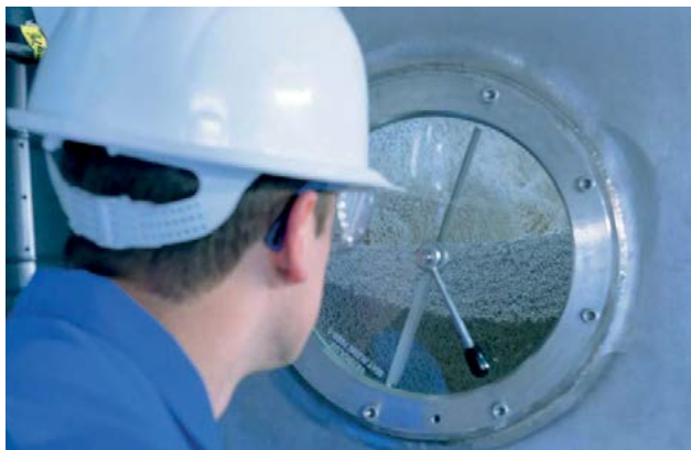
Fig. 4: The fluidised bed granulator is the centrepiece of the production plant.
