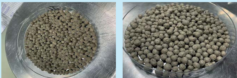
Figs 5 & 6: Single-layer moisture uptake test on calcium ammonium nitrate (CAN) granules. Results for untreated CAN (left) and anti-moisture coated CAN (right)
