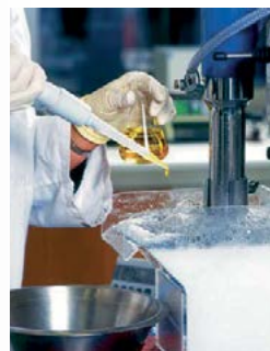
Cover: Laboratory benefication test with a Denver flotation machine. Nouryon.
