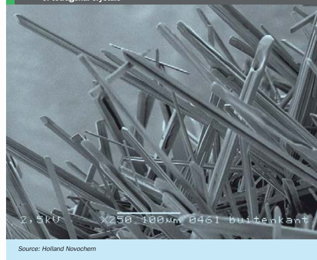
Fig. 2: Dust formation on the surface of urea granules due to the recrystallisation of tetragonal crystals
