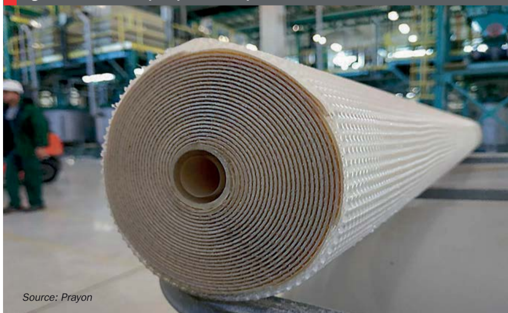
Fig. 4: Membrane for phosphoric acid purification
