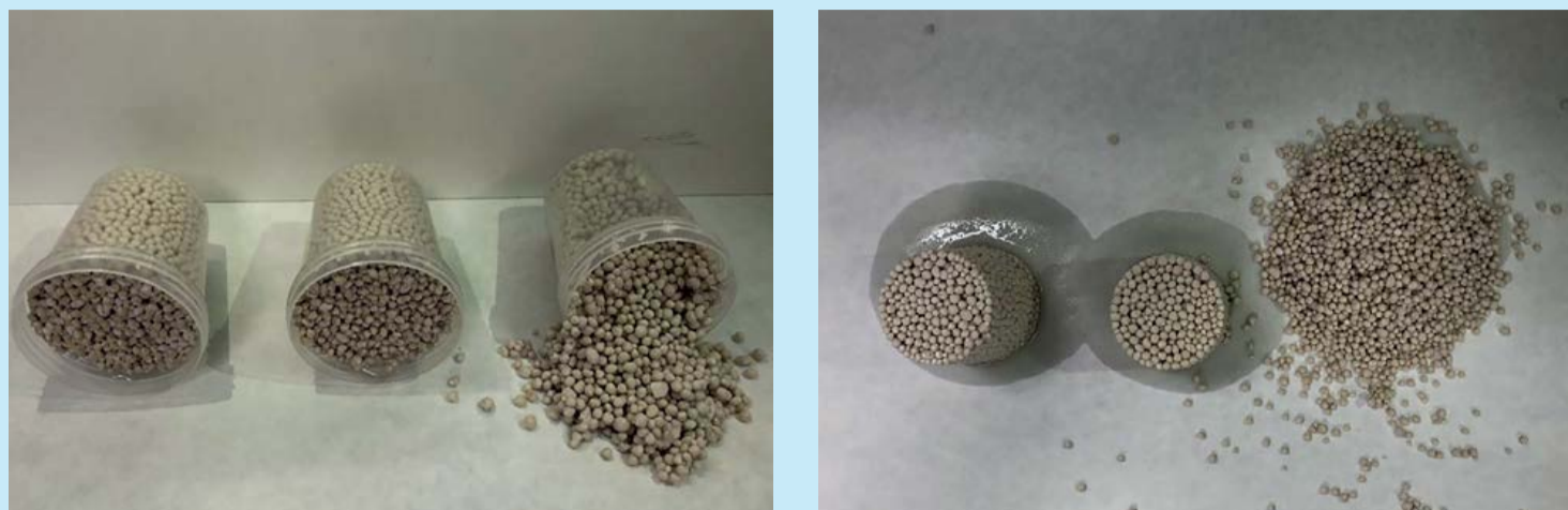
Figs 3 & 4: Moisture uptake test on calcium ammonium nitrate (CAN) granules. Results for (from left to right) untreated, anti-caking coated and anti-moisture coated samples
