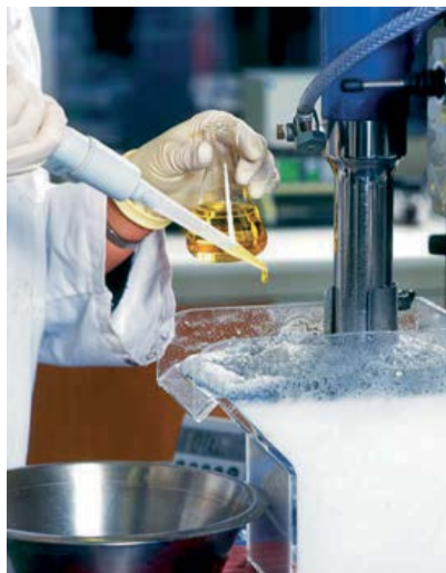
Cover: Laboratory beneficiation test with a Denver flotation machine. Nouryon.
