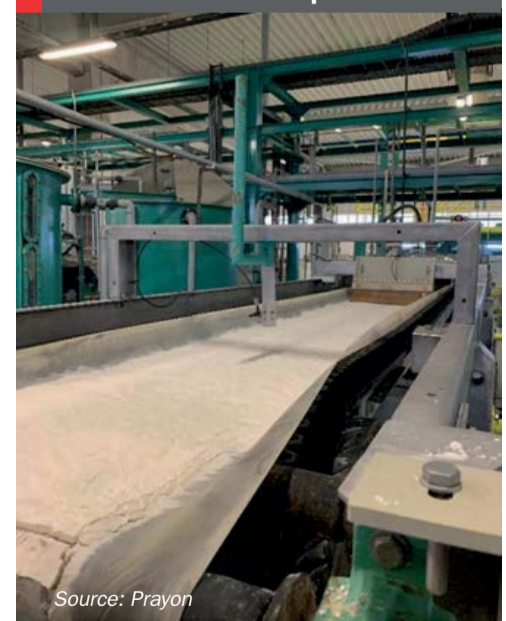
Fig. 7: Filtration at the Technophos semi-industrial plant
