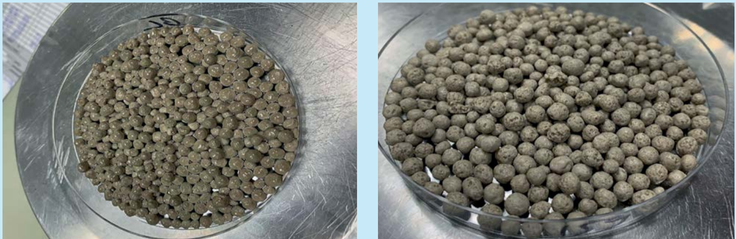
Figs 5 & 6: Single-layer moisture uptake test on calcium ammonium nitrate (CAN) granules. Results for untreated CAN (left) and anti-moisture coated CAN (right)
