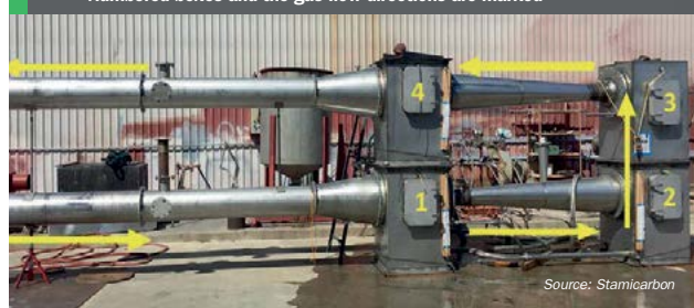
Fig. 6: Jet Venturi Scrubber pilot unit after fabrication in ECI's workshop. Numbered boxes and the gas flow directions are marked
