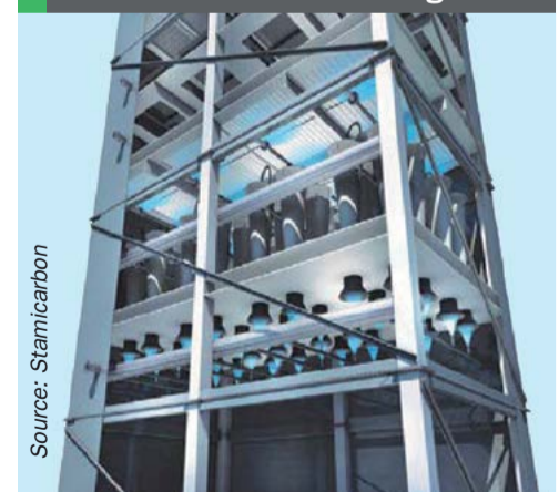
Fig. 3: New MicroMist™ Venturi Scrubber design
