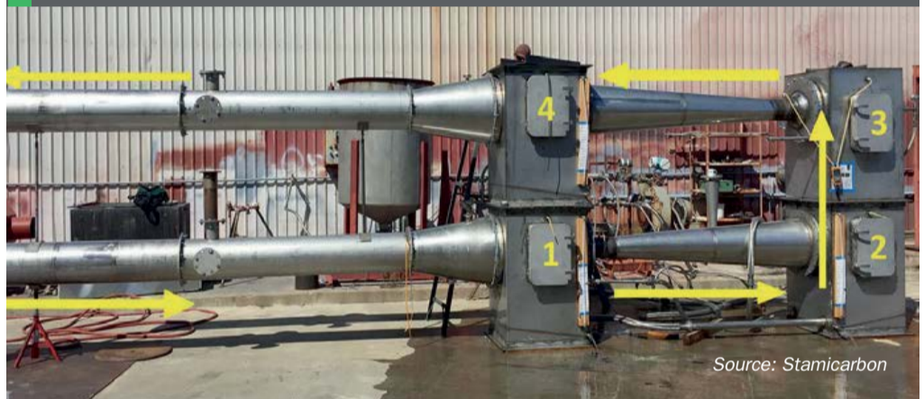
Fig. 6: Jet Venturi Scrubber pilot unit after fabrication in ECI's workshop. Numbered boxes and the gas flow directions are marked
