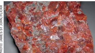
Permian-age potash-bearing rock, Carlsbad potash mining district, Eddy County, New Mexico. Potash ore needs to be crushed and ground to liberate the target mineral sylvite from unwanted halite.
