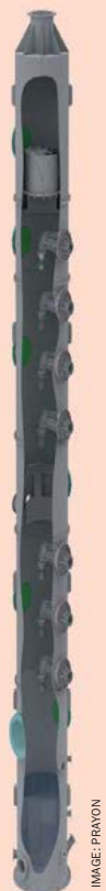
Fig. 2: Atmospheric gas cleaning tower. This system achieves under 5 ppm of fluorine in the waste gas.
