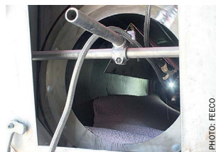
Fig. 5: Testing in a coating drum at the FEECO Innovation Center
