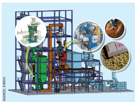
Left: Fig. 2: The Eirich SmartMixer. Right: Fig. 3: EIRICH SmartMixer within a fully automated mixing and granulation plant.
