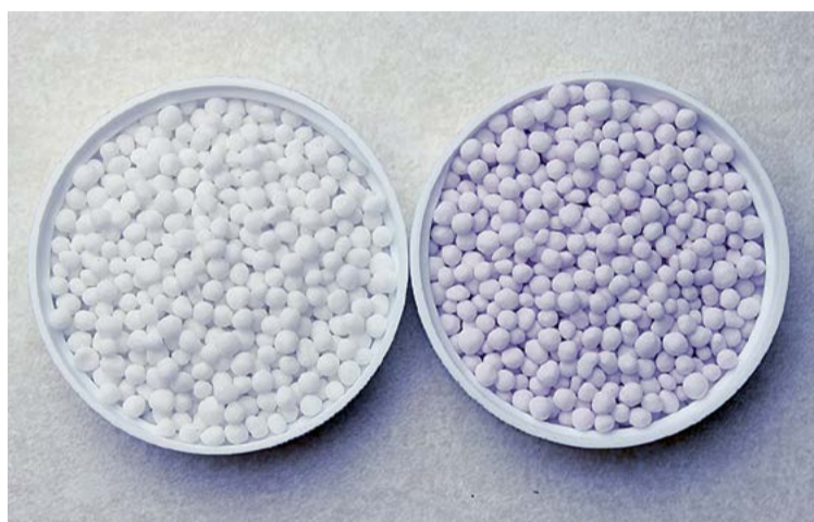
Fig. 2: Uncoated (left) and coated (right) urea granules. Urea is commonly coated to prevent moisture absorption from the air and subsequent caking.
