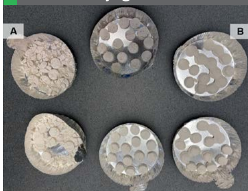
Fig. 1: Examples of incompatible binder-fertilizer interactions after drying
