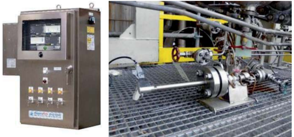
Fig. 7: Raman urea process analyser and special HP Raman probe.
