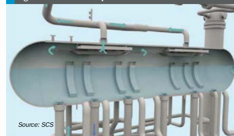
Fig. 3: Water steam separation in the steam drum
