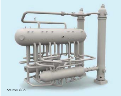
Fig. 1: Recommended heat recovery package arrangement
