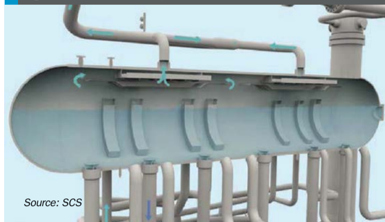
Fig. 3: Water steam separation in the steam drum
