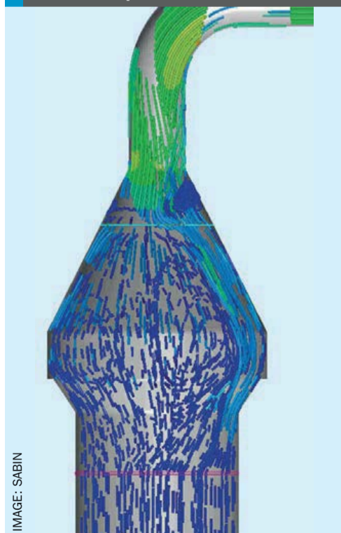
Fig. 13: CFD simulation with additional distribution plate
