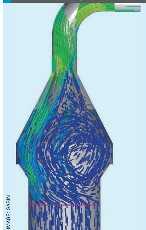
Fig. 14: CFD simulation with additional concentrically arranged truncated cones
