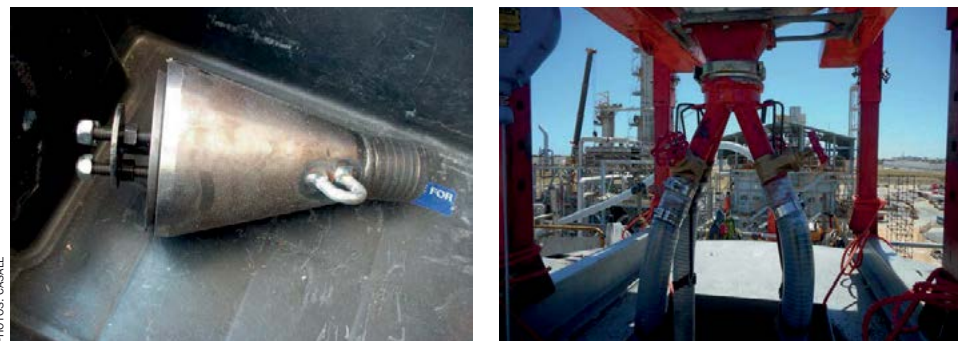
Above left: Fig. 1: Casale dense loading tool. Above right: Fig. 2: Detail of the fixed hopper on the converter top with details of valves for catalyst flow adjustment and hoses for catalyst feed.
