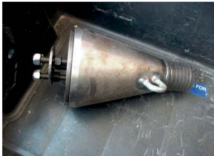
Above left: Fig. 1: Casale dense loading tool. Above right: Fig. 2: Detail of the fixed hopper on the converter top with details of valves for catalyst flow adjustment and hoses for catalyst feed.
