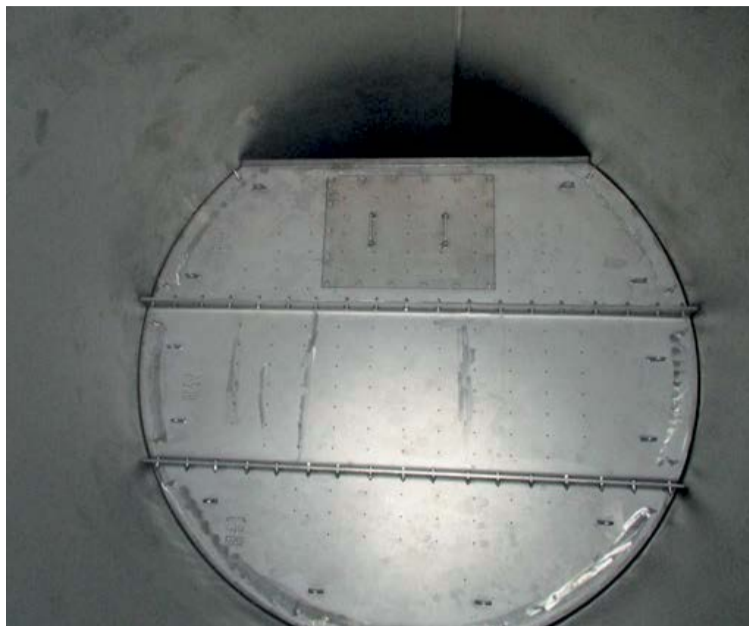
Fig. 3: Tray in SPIC reactor.
