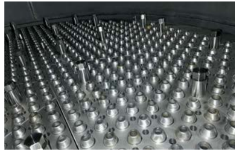
Left to right: HP Uremium29 stripper, Uremium29 components in the HP stripper top and Uremium29 tube to tubesheet orbital welding.
