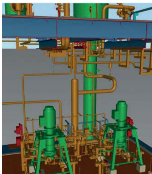
Fig. 1: Typical setup of a self-regulating pump.
