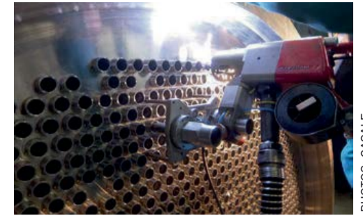
Left to right: HP Uremium29 stripper, Uremium29 components in the HP stripper top and Uremium29 tube to tubesheet orbital welding.
