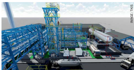
Module structure of a small-scale green ammonia plant from thyssenkrupp Industrial Solutions. Centre: ammonia synthesis; Right: pressurised ammonia storage tank.
